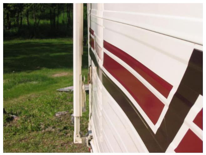
The above picture shows a bulge in the siding that indicates a delamination problem. The wall siding has separated from the Styrofoam insulation and a slight push on this area will show the extent of the damage. A bonded wall should be firm to the touch. The next picture shows the same area from another direction. Those lines are not straight!
