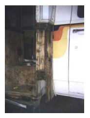
If the affected area is small and easily accessible, it may be possible to repair it from the inside of the coach, although it may be impossible to find an exact match for the paneling. If the area is in the bathroom, for example, a panel with a similar texture and color could be used with a border edge to separate it from the rest of the ceiling. If the area were in the living room section, a panel replacement would be very obvious.
