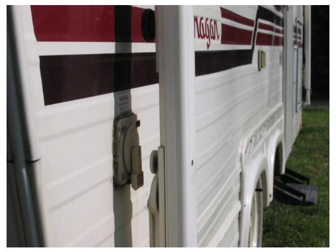
Delamination is very expensive to fix. The entire wall would have to rebuilt to repair the damage.
