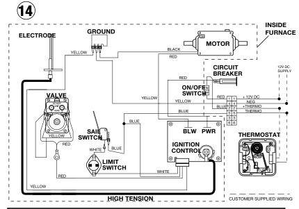
**IMPORTANT:** If any original wire has to be replaced, it must be replaced with type 105° C or its equivalent. Terminal Block on 85 Models only.
